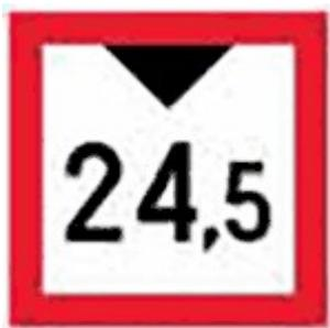
Figure 18. Restricted overhead clearance
