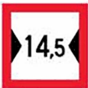
Figure 20. Limited width of passage
