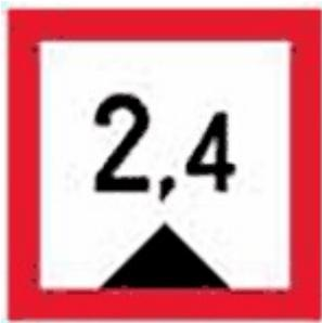
Figure 19. Limited depth of water
