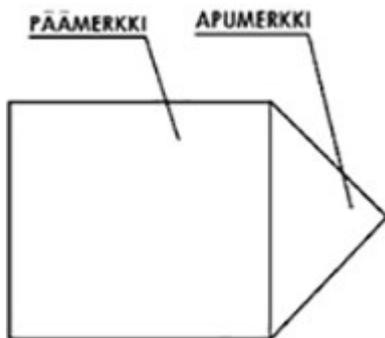
Figure 34a. Auxiliary sign indicating the effective direction of the main sign
